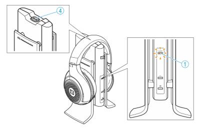
▶ Place the headphones on the headphone holder/charger of the transmitter. Make sure that the headphones make good contact with the charging contacts ④.
