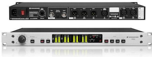
The design of the processing unit is clearly laid out with four directly selectable presets. If needed, these presets can be modified via an Ethernet interface. The processor software enables the user to adjust the gain of the individual channels, modify the front and surround focus, determine the surround delay, adjust several filters with their cut-off frequencies and set the compression, the limiter and the treble boost.
