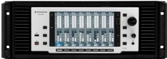
The modular EM 9046 receiver is a mainframe that accommodates up to eight receivers internally. The receiver system covers the UHF range from 470 to 798 MHz (328 MHz band-
