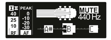
The **Guitar Tuner** standard display is deactivated upon delivery. To show this standard display, you have to activate it (see "Advanced -> Guitar Tuner menu item").
