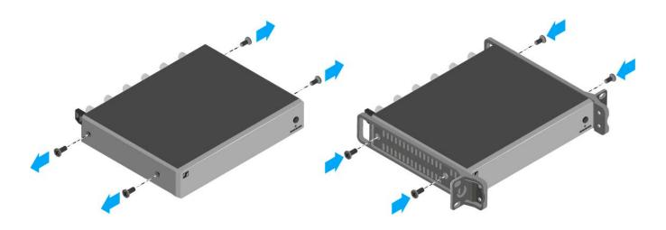
▷ Secure the blanking plate to one of the mounting angles using two recessed head screws (M6x10).
