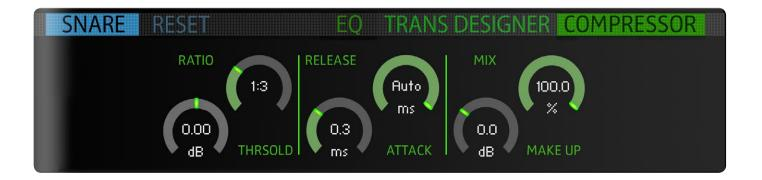
RATIO Controls the amount of compression, expressed as a ratio of "input level change" against "output level change". A Ratio of 1:1 means that no compression will be happening. For example, a Setting of 4:1 means for every 4 decibel increase of amplitude above the threshold, the output will increase by only 1 decibel.
