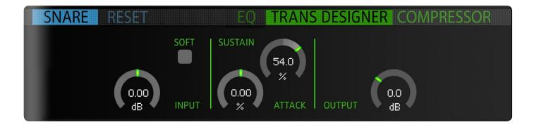
soft Trans Designer is designed mainly to work on drums or percussive material, so certain input signals (for example: an acoustic guitar) may not work ideally in the default mode, so try switching this button on if you are encountering problems.
