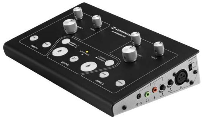
The SL Interpreter is a compact and stand-alone audio control center for simultaneous interpretation of one or more languages. It allows one or two interpreters to monitor floor or relay sources, activate microphone inputs, and route the interpretation signal to different outputs. Ideal for presentation-style conferences, where a floor and a single relay language are used. Recommended to be used with Sennheiser Tourguide 2020 or 1039.
